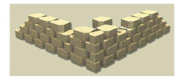
\*To split a block, use a hydraulic splitter or split manually by using a hammer and chisel to score the block on all sides. Pound the chisel on the same line until the block splits. If partial unit sides are not exposed, use a circular cut-off saw with a masonry blade to achieve a tighter fit.
